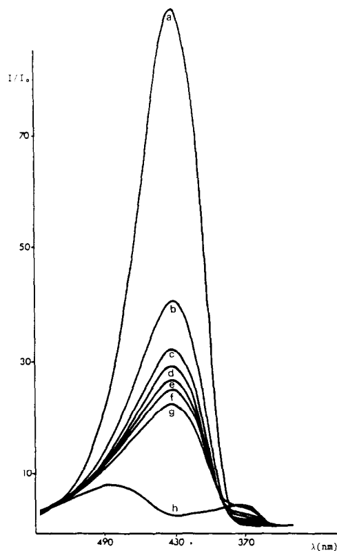
Fig. 8. Fluorescence spectrum of harmane ( \lambda_{\text{ex}} = 312.5 \text{ nm} ; concentration, 5 \times 10^{-5} \text{ M} ; ionic strength, 0.1): curve a, pH 1.00; curve b, pH 6.82; curve c, pH 7.24; curve d, pH 7.64; curve e, pH 7.82; curve f, pH 8.29; curve g, pH 13.00.
